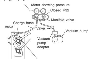
When pumping starts, slightly loosen the flare nut to check of air sucked in. Then tighten the flare nut.
